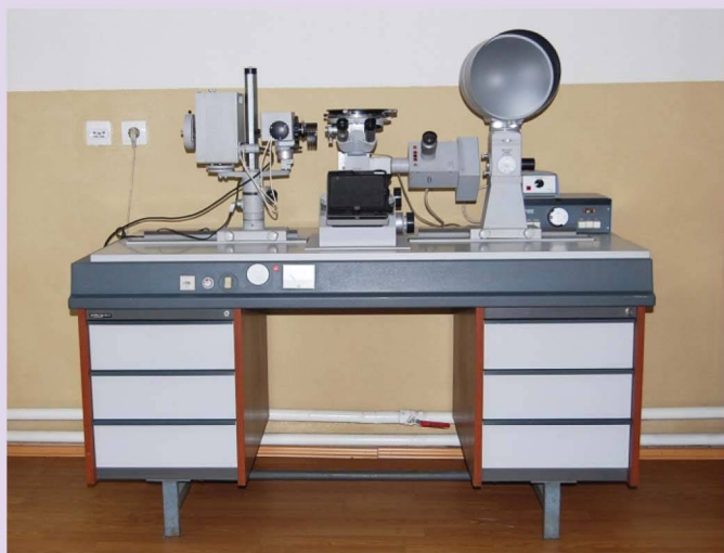
Metalografski mikroskop u laboratoriji Planita Metallographic microscope in the Planit laboratory
